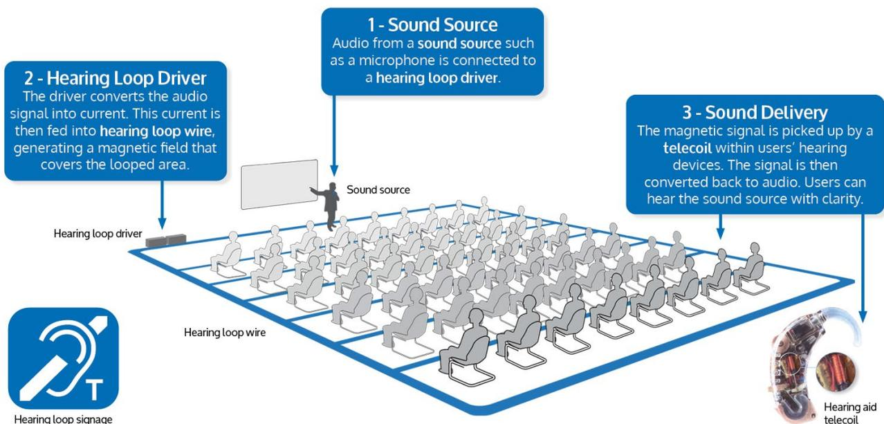
**Hearing loop systems provide better communication access by transmitting sound directly to telecoil-equipped hearing aids, cochlear implants or other assistive listening devices. (Graphic courtesy of Contacta & The HATGroup)**
